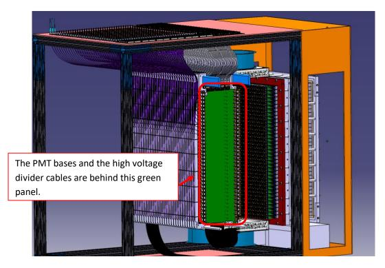
From [4]. Behind the green panel are the high voltage divider cables that connect to the PMT bases. What is unclear is what the other end of those cables are connected to and how they get connected to the patch panel on the roof interior.
